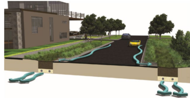
FIGURE 4 STREETScape WATER SENSITIVE URBAN DESIGN TREE PITS (WATER BY DESIGN, 2009)
