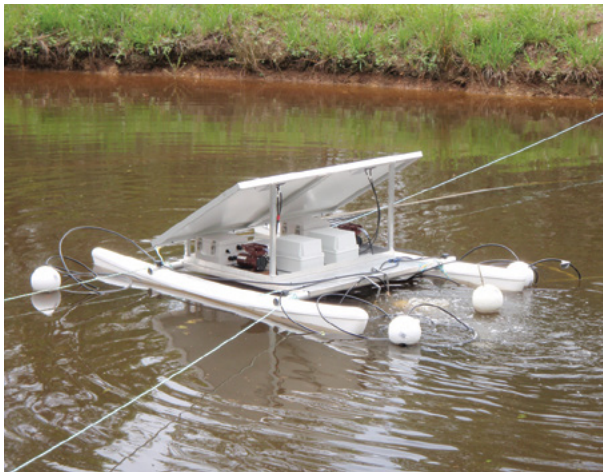
Figure 5.38 Solar water circulation system from behind
