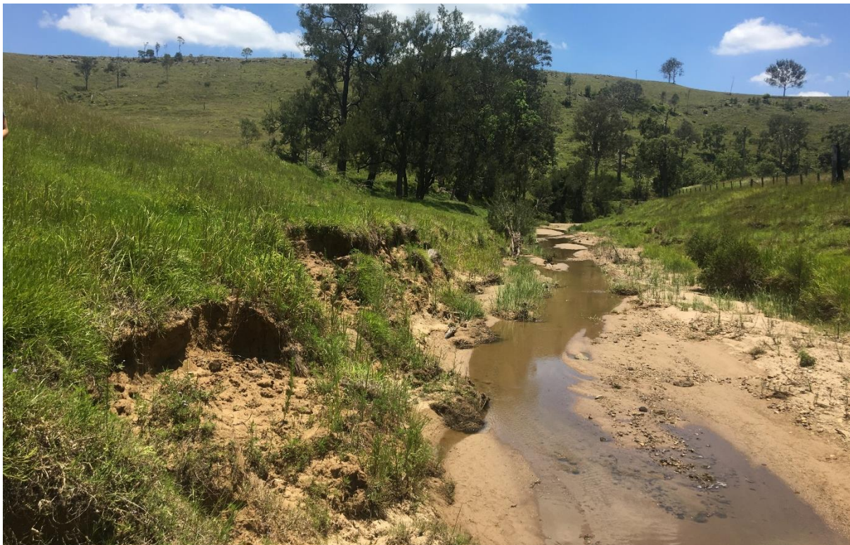
Figure 45. Knapps Creek – classified as significantly confined by floodplain/terrace with moderate instabilities of inset units between 2009-2016. Field verification indicated bank instabilities along the lower bank which comprised of inset benches and no lateral adjustment of macrochannel bank observed.
