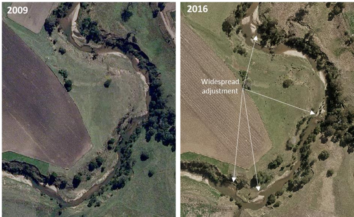
Figure 19. A section of the Logan River with major adjustment of inset units between 2009 and 2016
