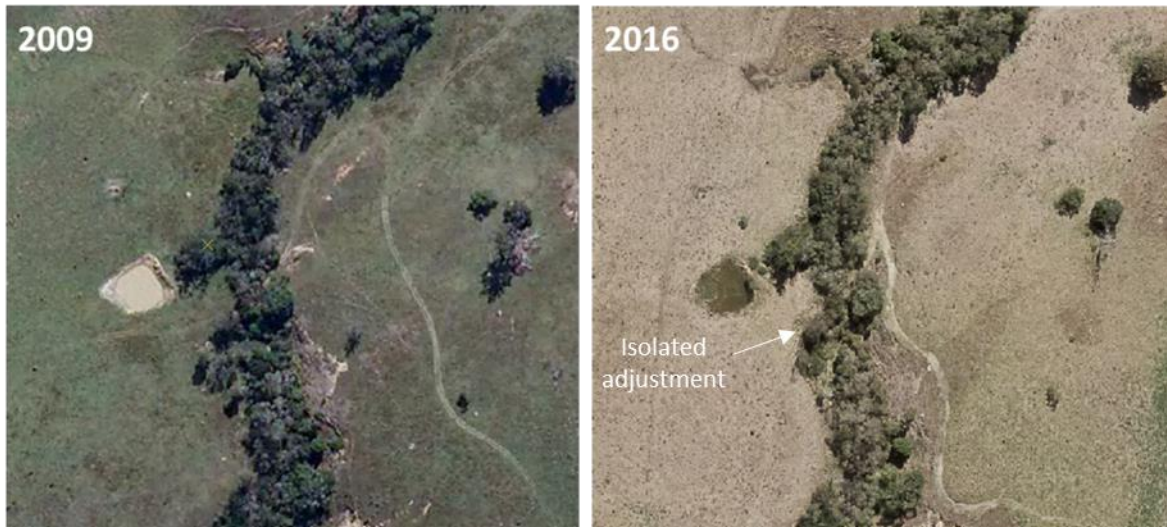
Figure 13. A section of Sandy Creek in the Logan River catchment with minor lateral adjustment between 2009 and 2016
