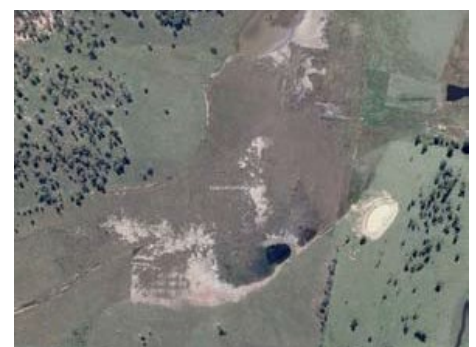
Image 1: Dams can have an impact on the water balance and result in rising water tables, concentration of salts and in severe cases bare ground which are more susceptible to erosion.
